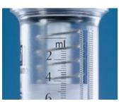
**Semi-automatic dispensing** The spring-loaded piston refills the cylinder after dispensing.
