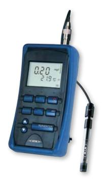
Lightweight and compact, these robust meters are both waterproof and submersible to IP 66/67.
