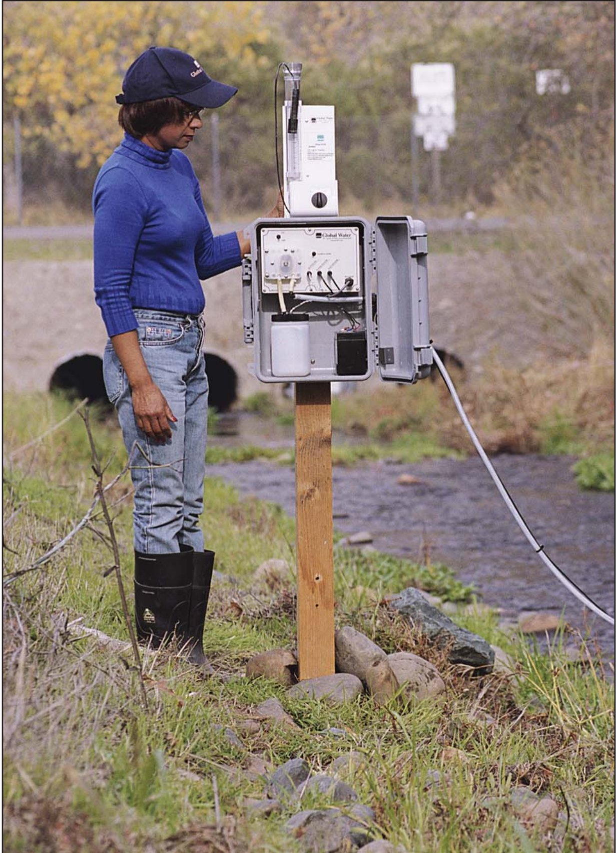
Monitoring stormwater runoff with a custom Global Water sampling system.
